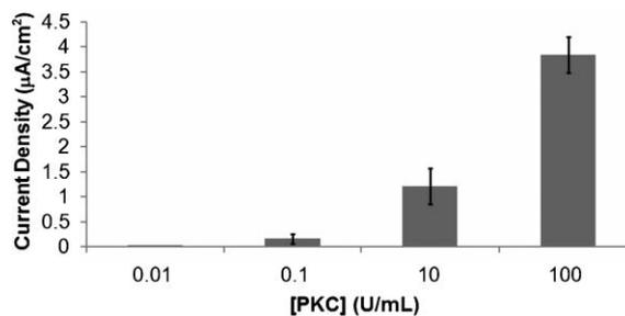
**Fig. 2** The dependence of current density responses on the concentration of PKC obtained from the cyclic voltammetric data. The error bars indicate the standard deviation ( $n = 3$ ). Other experimental conditions were as described in Fig. 1.
