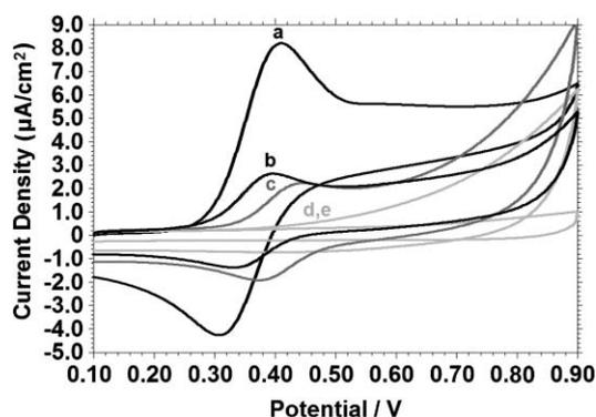
**Fig. 4** Cyclic voltammograms for the PKC-catalyzed phosphorylation reactions in the presence of 100  $\mu\text{M}$  Fc-ATP and 100  $\text{U mL}^{-1}$  PKC at varying incubation periods at 30  $^{\circ}\text{C}$ , (a) 1 h, (b) 20 min, (c) 10 min, (d) 5 min and the electrodes were not incubated in the assay solution (e). Other experimental conditions were as described in Fig. 1.
