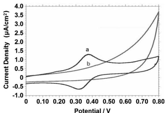
**Fig. 1** Cyclic voltammograms for the PKC-catalyzed phosphorylation reactions (a) in the presence of  $10 \text{ U mL}^{-1}$  PKC with  $100 \text{ }\mu\text{M}$  Fc-ATP, (b) in the absence of PKC. Kinase assay solution also included  $20 \text{ mM}$  Tris,  $0.5 \text{ mM}$  EDTA,  $10 \text{ mM}$   $\text{MgCl}_2$ ,  $500 \text{ }\mu\text{g mL}^{-1}$  phosphatidyl serine (pH 7.5). Measurements were taken in  $0.1 \text{ M}$   $\text{NaClO}_4$  solution at  $100 \text{ mV s}^{-1}$ .
