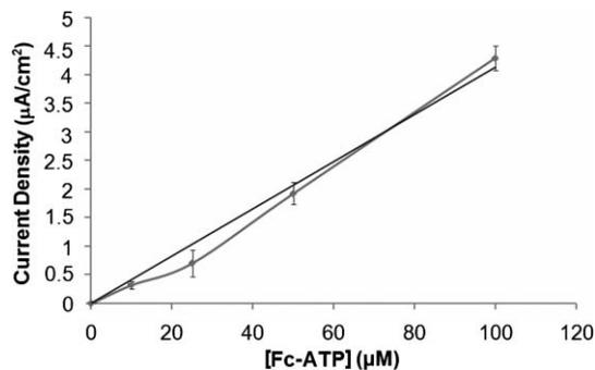
**Fig. 3** Plot for the dependence of current density responses on the concentration of Fc-ATP. Other experimental conditions were as described in Fig. 1.
