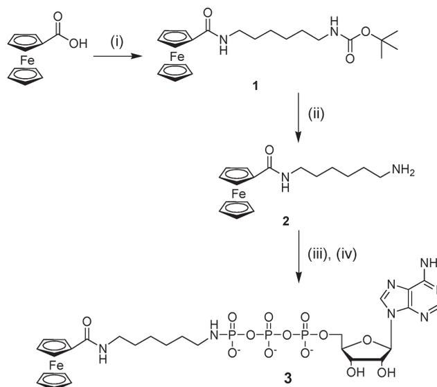
**Scheme 1** Preparation of the Fc-ATP conjugate **3**. Reagents and conditions: (i) TEA, HBTU, BocNH(CH<sub>2</sub>)<sub>6</sub>NH<sub>2</sub>; (ii) (a) TFA, DCM, (b) TEA; (iii) ATP, DCC, DMF; (iv) compound **2**, MeOH.
